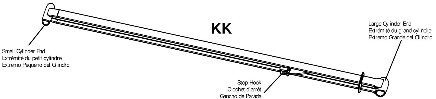
17. Rotate the Lid Support Prop Rod (KK) so that the small cylinder end will pass through slot in the top front of Upper Side Panel (CC or EE as Prop Rod can be placed on either right or left side).
