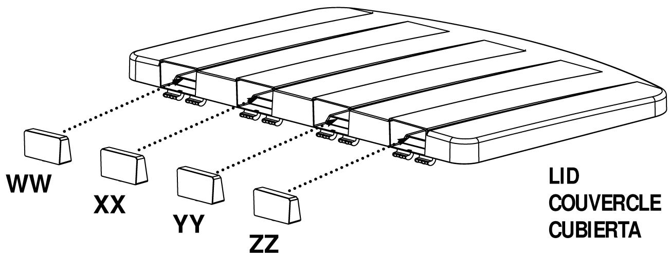
15. Assemble Lid by taking Lid End Caps (WW, XX, YY, ZZ) and pushing them into the respectively marked openings in the Lid.
