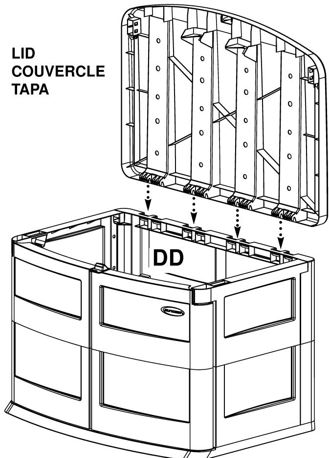
16. Hold Lid in an up / open position parallel with the Upper Back (DD) then hook the Lid hinges to the Upper Back hinge receptacles. Carefully close Lid to engage.
