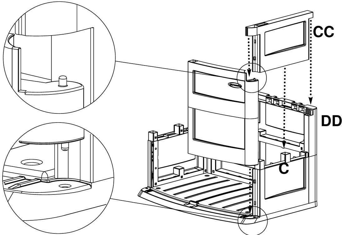
11. Place right door assembly by positioning the door peg (which protrudes from the Lower Door Cap) into the door peg receptacle located in the Base.
