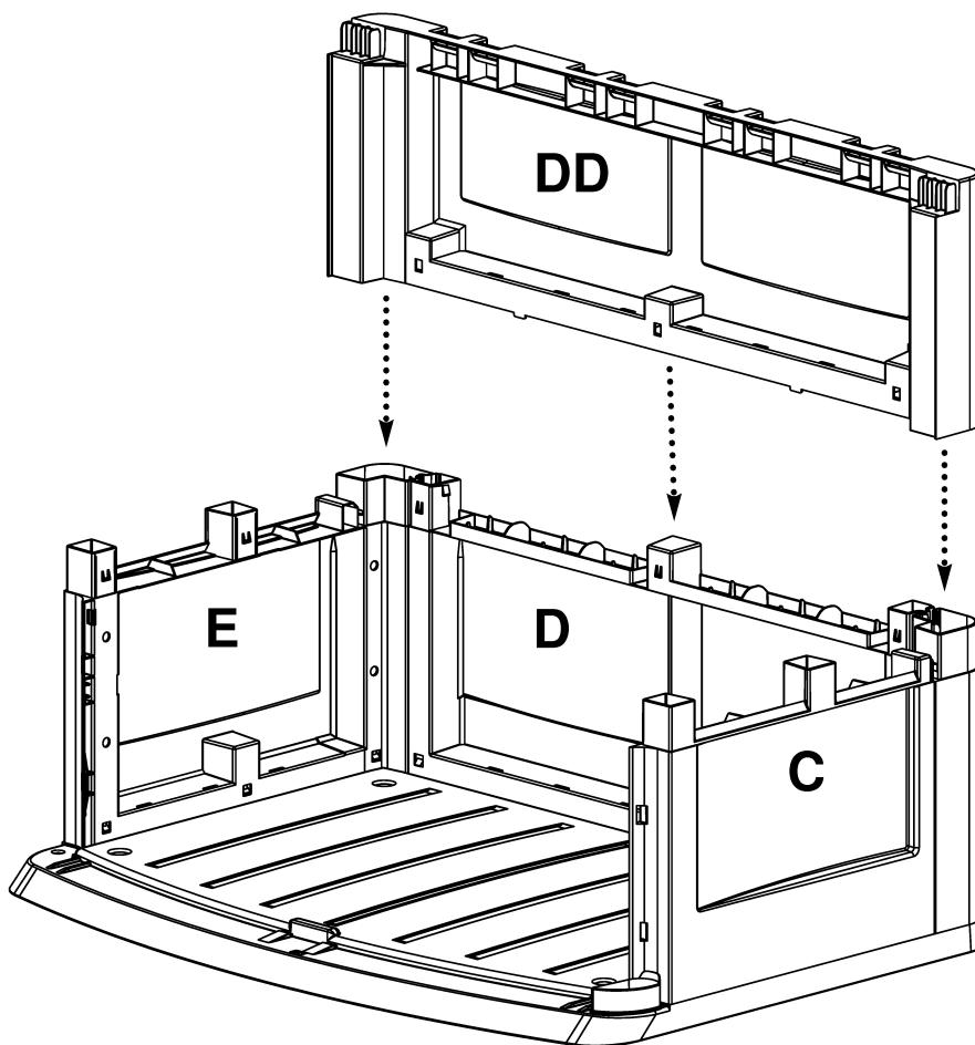
10. Place Upper Back (DD) onto Lower Back (D) making sure to connect to Lower Sides (E,C). Press down until Upper Back snaps into place.
