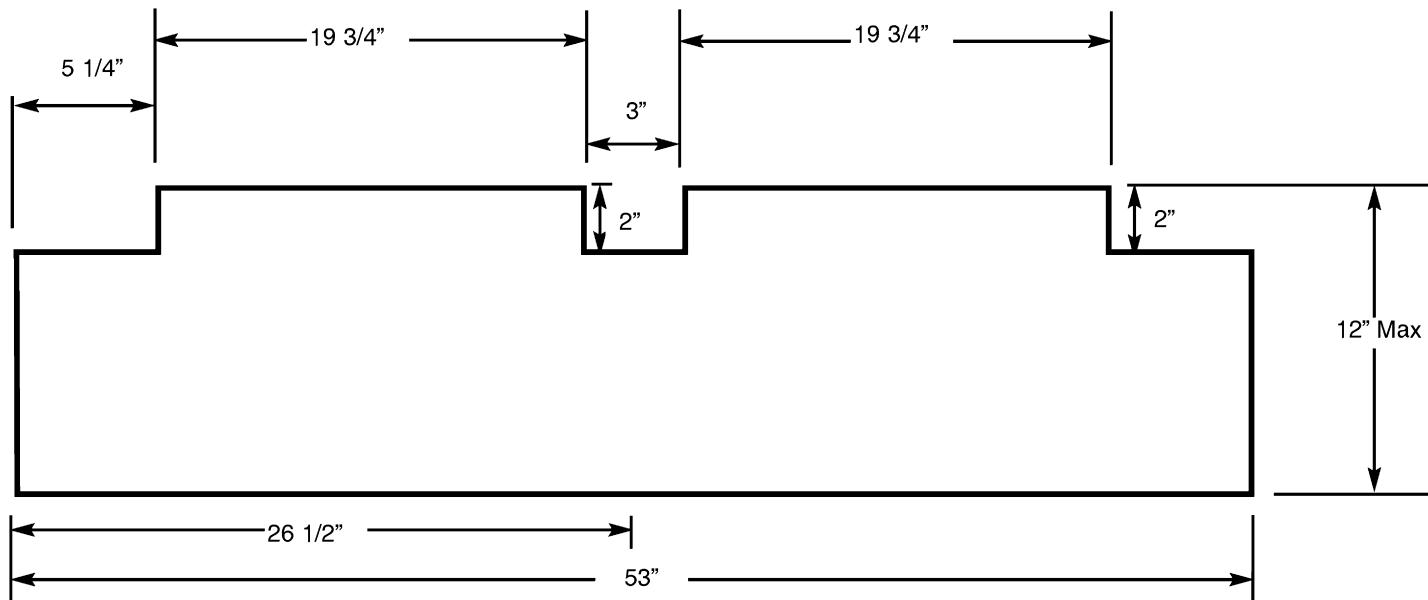
**Shelving:** Shelving can be added to your Suncast storage shed by utilizing the provided dimensions and cutting your own shelf from 1" thick shelving material. The notched corners face the back of the shed and fit into the inner shelf brackets that have been molded into the inner sides of your storage shed.
