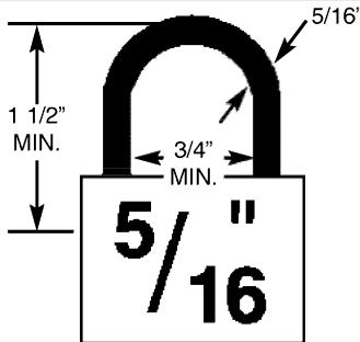
**Securing Your Shed:** To properly lock your shed using the Padlock Assembly feature, 5/16" padlock is recommended.
