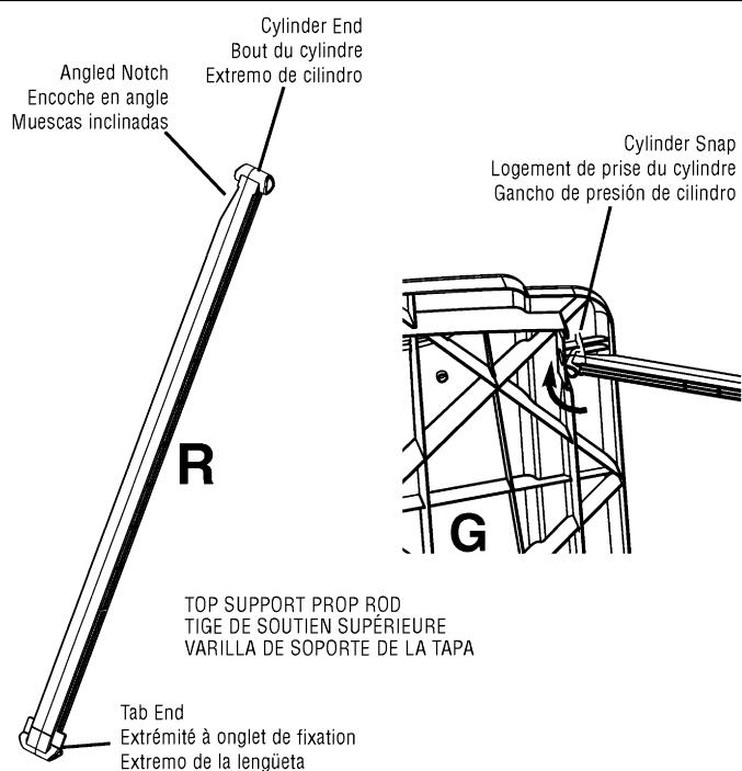
14. With cylinder end attached to Top (G), twist the tab end of the Prop Rod (R) so that it will pass through slot in the top front of Side Panel and then untwist.
