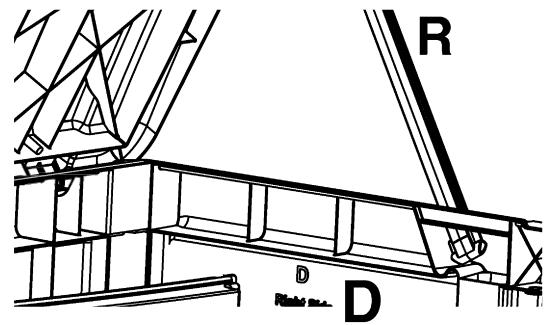
15. To use Prop Rod (R) feature, open Top (G) to the point where the prop rod lifts and sets in the prop rod receptacle.
