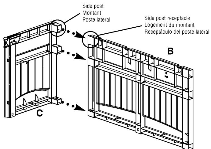
3. Attach Right Side Panel (D) to Back Panel (B) as done in step 2. Press parts together until pieces snap in place.
