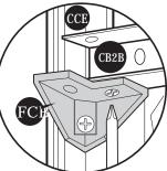
Fig.4: Use (S1) screw. Fix (CB2B) to (FCB).
