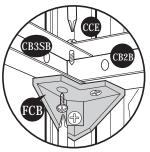
Fig2: Use (S1) screws. Fix (CB3SB) to (FCB) and (CB2B).
