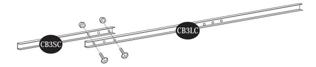
8. Assemble the center bands (CB3SC) & (CB5C) with (S3) screws with nuts. Fix (FCB5C) to (CB5C) with (S3) screws with nuts. Follow overlapping method shown below.
