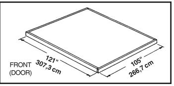
Note: Finished Slab dimensions, with lumber removed.
