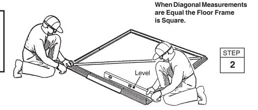
The floor frame *must be square* and level or holes will not align.
