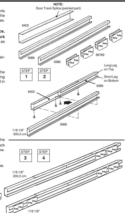
**3** Position **door slides** onto the legs, from the end of door track assembly, as shown in the end view.
