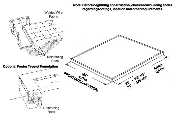
Note: Finished Slab dimensions, with lumber removed.
