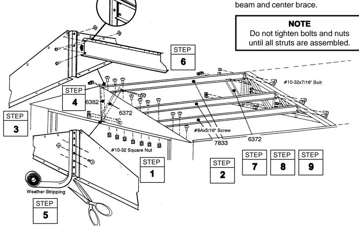
● Parts Needed For ● Step 17 Roof Beams 12x17, 12x24 & 12x31 <sup>BW29</sup>
