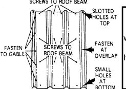
If roof beam holes do not line up with the roof panel holes, shift the building from left to right. If this does not help, your building may not be level. Shim the corners until holes line up.
