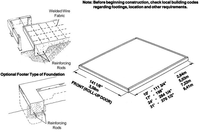
**Note:** Finished Slab dimensions, with lumber removed.
