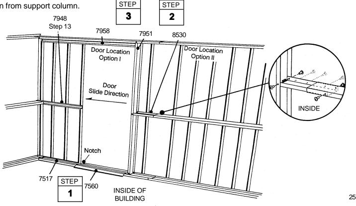
• 7946 Door Jamb (2) **7948 Door Wall Brace (1)** Step 13 Parts Needed For • 7972 Door Handle Lock Bracket (1) Side or Rear Entry Door All Sizes BW26
