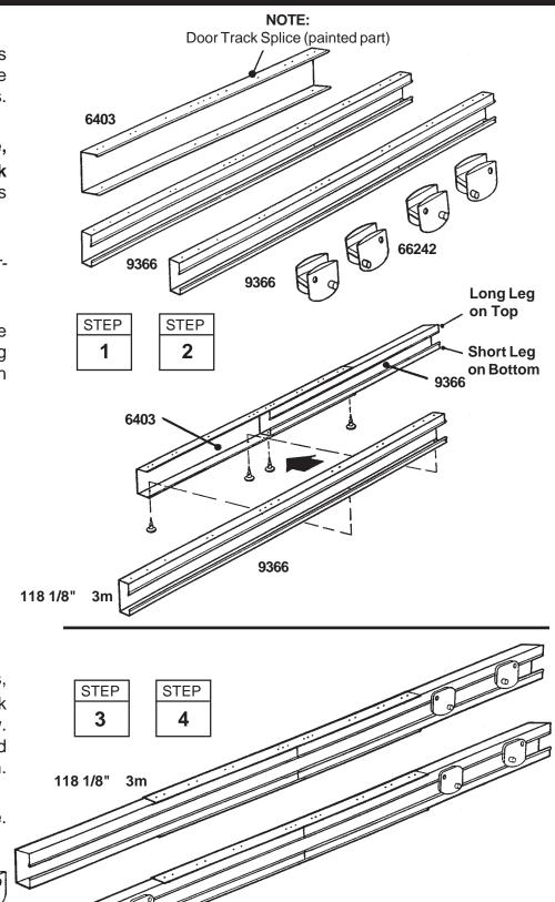
**3** Position **door slides** onto the legs, from the end of door track assembly, as shown in the end view. NOTE: Flat side on top, pins and holes <u>must</u> be oriented as shown.
