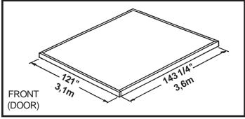
Note: Finished Slab dimensions, with lumber removed.
