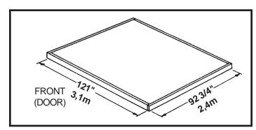
Note: Finished Slab dimensions, with lumber removed.
