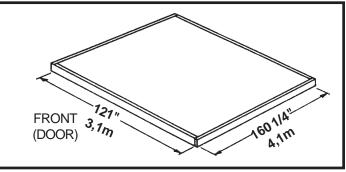
Note: Finished Slab dimensions, with lumber removed.
