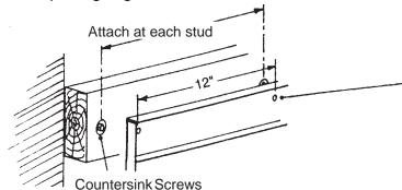
Note: Poke a hole through weather seal using an awl before drilling or fastening.
