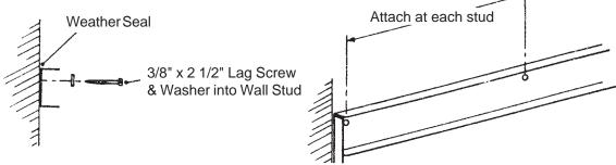
**Option 2 Attachment to Brick or Masonary** Use masonary fasteners (purchased locally) 12" on center. **Level** rear roof channel on wall, using holes in rear roof channel as a guide, drill holes in wall at the center and each end of channel with proper size masonary bit ( do not drill holes in mortar joints). Attach rear roof channel to wall with masonary anchors. Repeat procedure for remaining holes in rear roof channel for attaching to wall.
