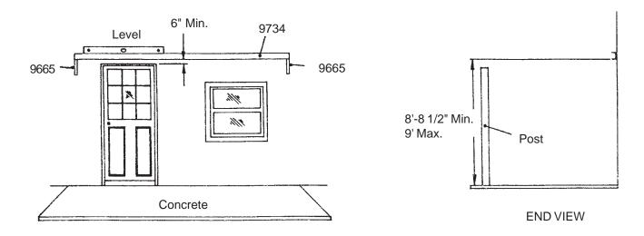
**2 Channel Weather Stripping** Attach weather stripping 1/2x 1 1/2 to one end, on the outside of rear roof channel. Making sure weather stripping is flush with top flange of rear roof channel, continue to stick weather stripping to rear roof channel. Peel paper backing.
