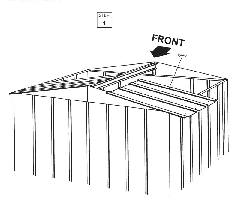
Parts Needed For Front of Roof
