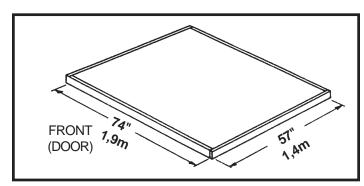
Note: Finished Slab dimensions, with lumber removed.
