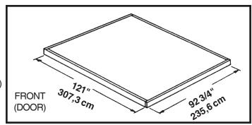
Note: Finished Slab dimensions, with lumber removed.
