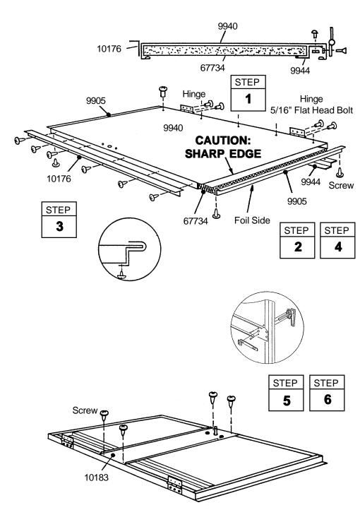
● Parts Needed For ● **Left Door Assembly**  9905 Door Brace (2)
