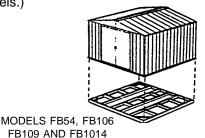
A simple new floor frame system that works as a foundation. Self-Squaring, made of heavy-duty, hot-dipped galvanized steel. Use as foundation for plywood, pour concrete, sand or stone.
