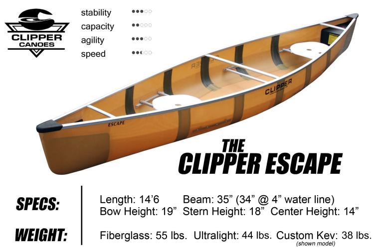
The Escape is great for fishing, photography, or bird watching. The comfortable seats allow paddlers to sit instead of kneel. It has a near vertical bow and stern to aid in tracking. The Escape's short length allows it to maneuver easily in tight spots and its very manageable weight makes the Escape easy to load and transport.
