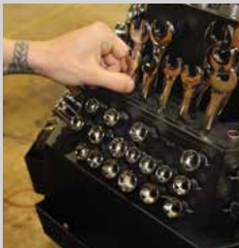
Foam inserts store and organize your tools. Steel tines keep frequently used sockets at hand.
