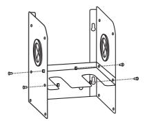
Attach the two side panels to the top shelf using two bolts and nuts per side.
