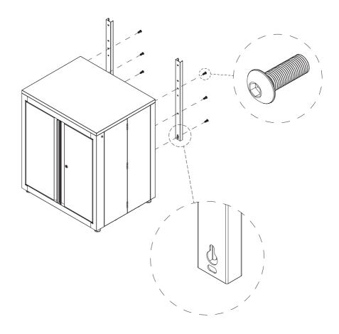
Slide two B posts fully onto the A posts.
