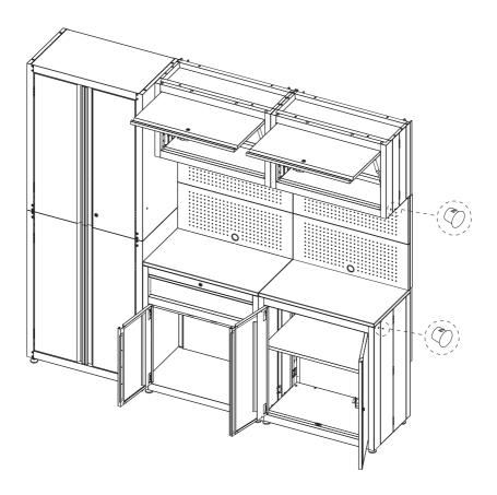
For safety, secure the tops of the each unit to the wall using M6 x 65 mm hex tapping screws and washers. Use three M6 x 65 mm hex tapping screws and washers on wall cabinets and three M6 x 65 mm hex tapping screws and washers on base cabinets.
