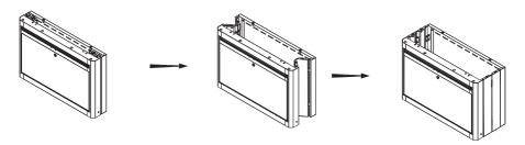
Insert the lip of the bottom panel into the slot in the back of the cabinet, then tilt the bottom panel down. Make sure the holes are aligned.
