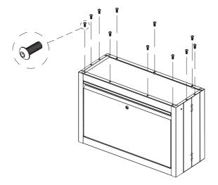
Turn the cabinet back to the upright position. Attach the top panel using eight M6 x 16 mm hex socket head screws.
