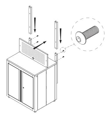
Slide two A posts onto the B posts. Make sure to leave enough room at the top for the wall cabinet.
