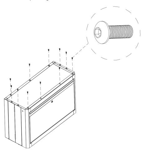
Turn the cabinet back to the upright position. Attach the top panel using eight  $M6 \times 16$  hex socket head screws.
