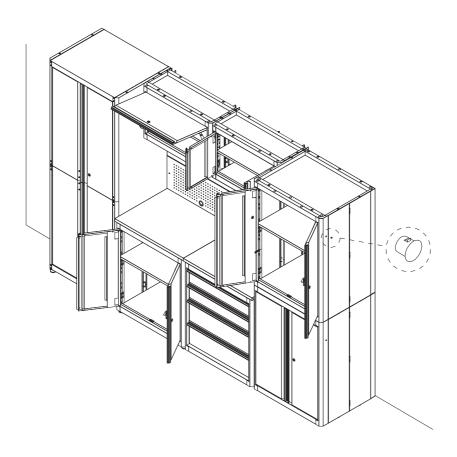
For safety, secure the tops of the each unit to the wall using three M6 x 65 hex tapping screws and washers.
