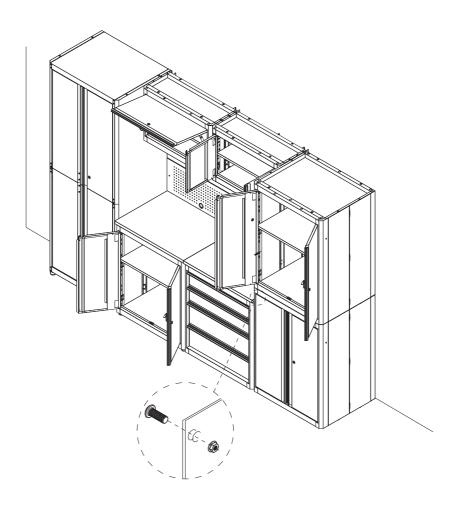
Hide holes on the exterior ends of the units with the supplied end covers, if necessary.
