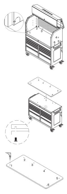
Take the hutch off the cabinet. Remove the worktop by first removing the drawers, then loosening the M6 x 12 Phillips head bolts.
