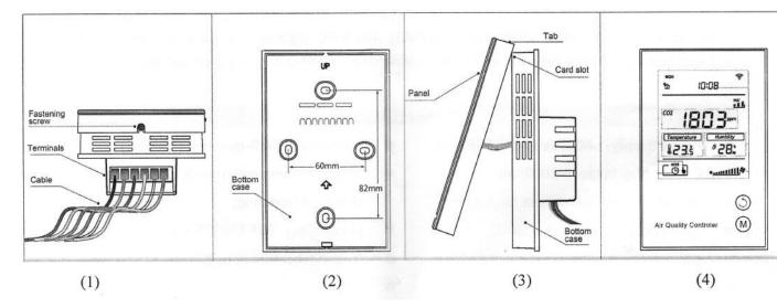
Step 1: Separate Panel and Bottom case by removing the screw at the bottom of device. Insert all wires into the right terminals and tighten screws. The wiring diagram is shown above
