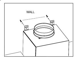
4. Secure and tighten the mounting screws.
