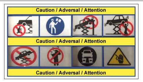
Attention 1 It is not allowed to stay under the vehicle, while operating the lift.
