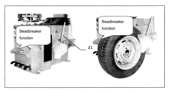
Fig 6. Separating the tyre
