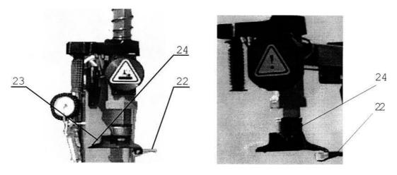
Fig. 7. Foot parts: 22-support, 23-bulb, 24-shoe
