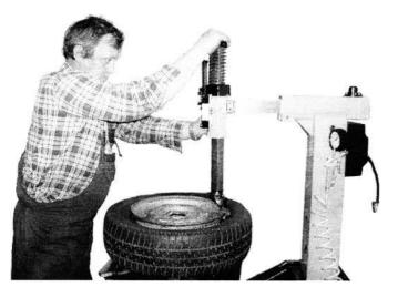
Fig. 8 Setting working head
