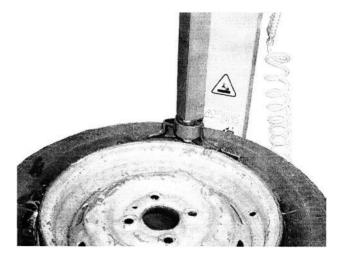
Fig. 9. Foot in operating position
