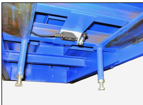
Picture 25 (lower limit switch)
