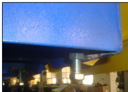
Picture 30 (adjustment screw)
