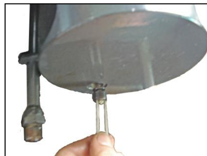
Picture 9 (antiknock valve)
