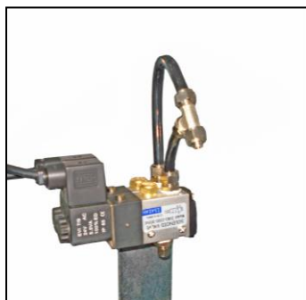
Picture 21 (solenoid air valve)
