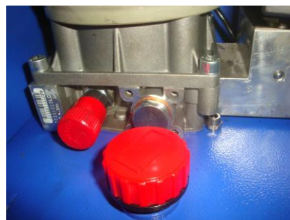
Picture 31 (oil tank)
