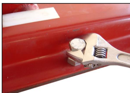
Picture 29 (adjustment bolt)
