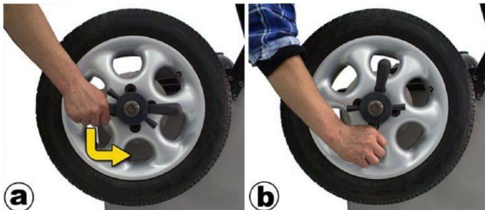
Fig. 9: Removing wheel from the holder.
