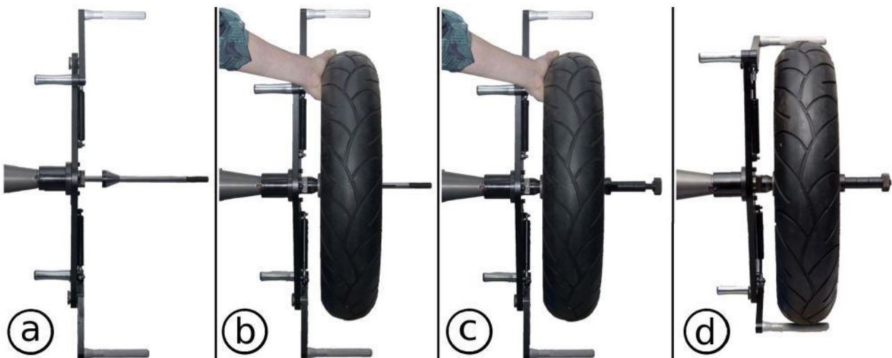
Fig. 14: Motorcycle wheel mounting on the holder.
