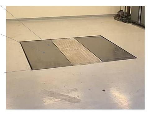
Scissor lift JA6001S is the perfect solution if you want a scissor lift in high professional quality. The lift is in-ground installed and the minimum height is only 11 cm. which makes the installation preparation minimal.
