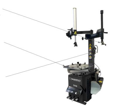
DWB+ is semi-automatic, suitable for cars, motorcycle and light truck. 20" turnable and powerful motor.
