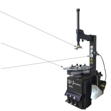
DWB is semi-automatic, suitable for cars, motorcycle and light truck. 20" turnable and powerful motor.
