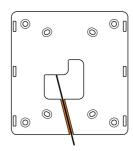
For on-wall cable installations only, route cable through highlighted channel.
