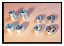
Starting From Top Left. 2. 7/8-3/4 Spacers (installed in pitman arm heim). 2. Thick 3/4 Spacers. 4. Thin 3/4 Spacers.
