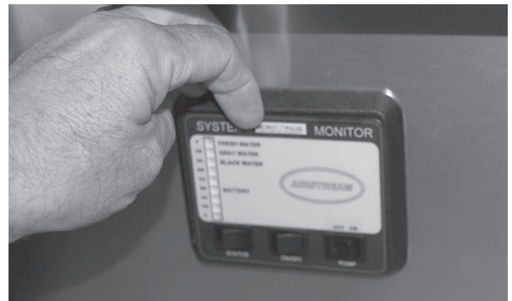
Fig. 4. To remove face panel of tank monitor, place fingernail between faceplate and bezel and pull out. (Faceplate is held by two clips along its bottom edge.)
