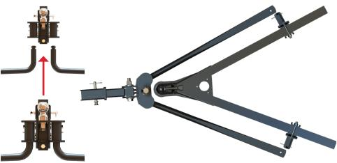
The optimal load on the Spring Bars depends on a combination of the Ball Mount tilt angle and the L-bracket height. Look at the distance from the bars to the bottom of the L-bracket. This should be 3" based on the previous setup instructions. If the distance is greater than 3", remove spacer washers until you have 3". If the distance is less than 3" add spacer washers until you have 3".
