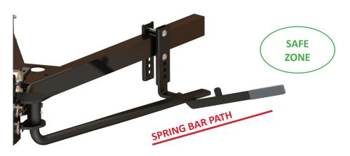
**WARNING:** Spring Bars under tension can kick back and cause serious injury. Stay out of the Spring Bars path until Safety Cover with R-Clip installed.
