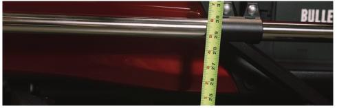
Measure from the ground to the bottom of the tube. You must have a minimum of 3'' to 4'' of clearance under the flaps.
