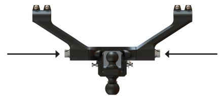
Tighten the bolts on both sides with the 1-1/8'' wrench. If you have a torque wrench torque to 85 ft-lbs.
