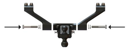
Note: Angle the position of the arms depending on the type of vehicle, and the bumper configuration.
