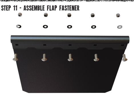
Place the flap on a flat surface with the smooth side facing down. Slide the mounting bracket over the flap with the square holes facing down. Place the carriage bolts into the hole from underneath the bracket, so the head of the bolt is facing the flat surface. Start with 1 bolt on each end and then continue with the middle bolts. Place the washers over the bolts, followed by the lock nuts. Hand-tighten the bolts until snug. Repeat these steps for the other flap.
