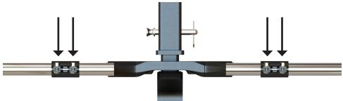
Tighten all four bolts evenly with the 1/2'' wrench. If you have a torque wrench torque to 12 ft-lbs.
