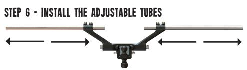
Slide the pole into the assembly and line up the end of the pole 1'' past the outside of the rear tire. Repeat this step for the other side.
