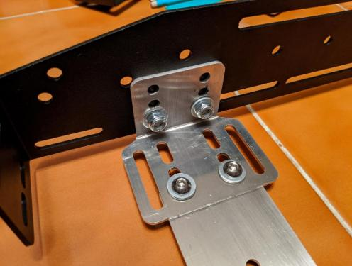
Do the same for the top of the side bracket. Leave this bracket extra loose as it will need to be slid up or down based on the size of your tire.
