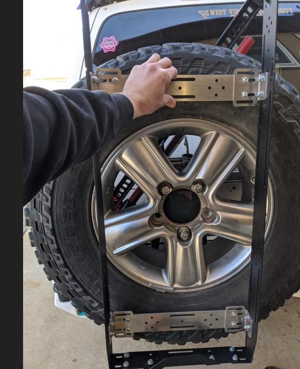
Now you can assemble the 4 front brackets. Use the same measurement method from earlier steps to ensure they are the same width as the back brackets.
