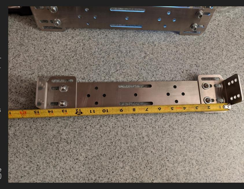
Attach one of the assemblies in the previous step to the lower portion of each side bracket as shown. The best starting point is the lowest slot position on the side bracket and the closest bolt holes to the 90-degree bend on the strap bracket. That's what's shown here. Note the position of the hardware. Nuts facing inward = better aesthetics. Bolt heads facing inward = easier removal of the tracks. I prefer the nuts facing in as shown. The tracks are still easy to remove.
