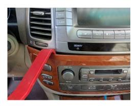
1) Use an interior plastic pry bar to remove the fascia around the tape player
