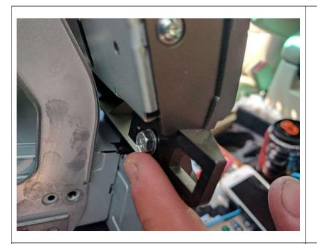
7) Remove the 2 bolts holding the tape deck to the navigation unit
