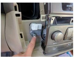
4) Remove the 4 bolts holding in the navigation and tape player. Slide the entire unit out enough to expose the plugs in the back of the unit
