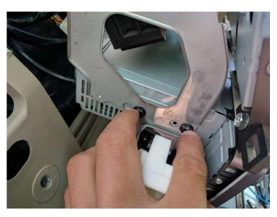
6) Remove the 4 bolts holding the tape player in place on the metal frame
