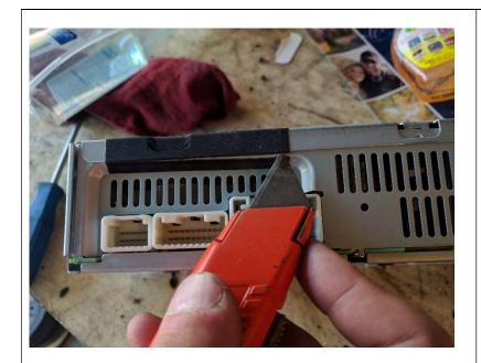
9) Cut the tape on the backside of the tape deck, then gently pry the lid of the tape deck revealing the inside
