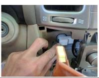
2) Remove the center differential, hazard lights, and airbag indicator plugs from the fascia and set it aside
