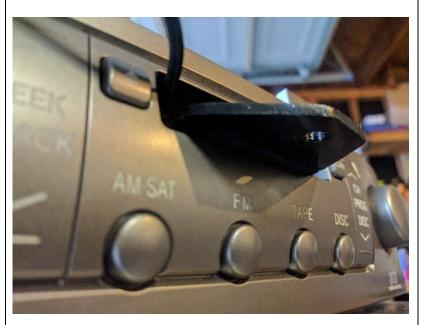
12) The tongue and its foam pad should rest snuggly against the bottom edge of the tape deck slot as show. This is important for stability and strength
