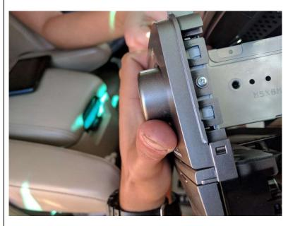
8) Slightly pull the tab seen in the bottom of the photo to separate the tape deck from the lower row of buttons. The tape deck should be completely removeable at this point
