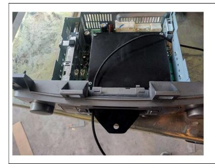
11) Install the Owl **Expedition Media** Mount using the 4 small screws, ensuring the tongue is sticking out of the tape deck slot. Now is a good time to run a charger if you intend to. Cutting or drilling a small hole in the cooling grates of the tape player works well. Ensure where you run the wire will not interfere with reinstallation
