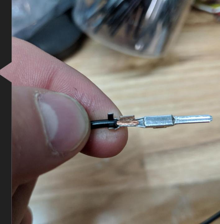
Using needle nose pliars, fold the clasps over onto the wire and insulation as shown.
