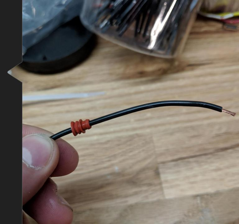
• Place conductor on the wire end as shown. Ensure the rear clasps are on insulation and not bare wire.
