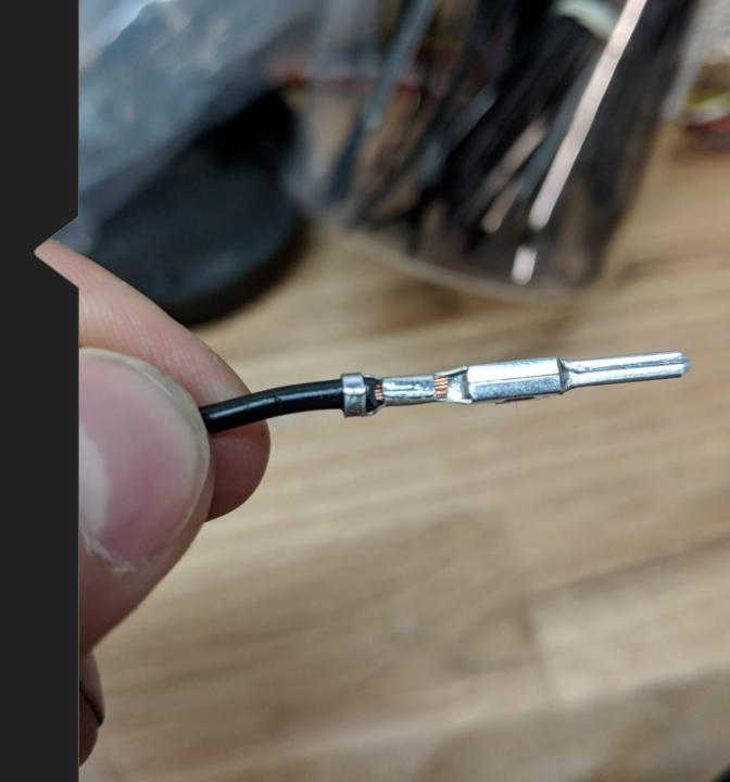
Using a wire crimping tool, crimp the forward most clasp onto the bare wire to ensure a secure connection. Soldering the wire to the conductor is also recommended, but not required.
