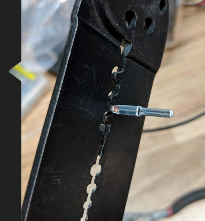
• Slide the rubber seal up over the first claps to where the second clasp begins, as shown.
