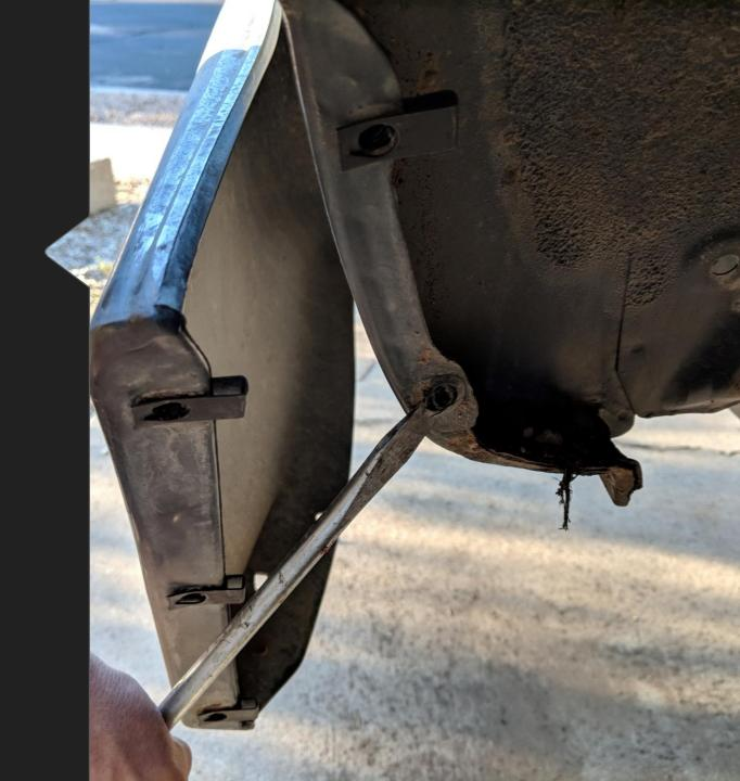
Using 3 flat head bolts, attach the stock rear bumper bracket to the rear bumper.
