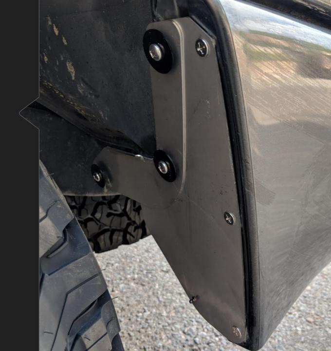
Remove the 3 bolts holding the front fender liner and cladding (LX470). Retain the bolt circled in yellow as it will be reused.
