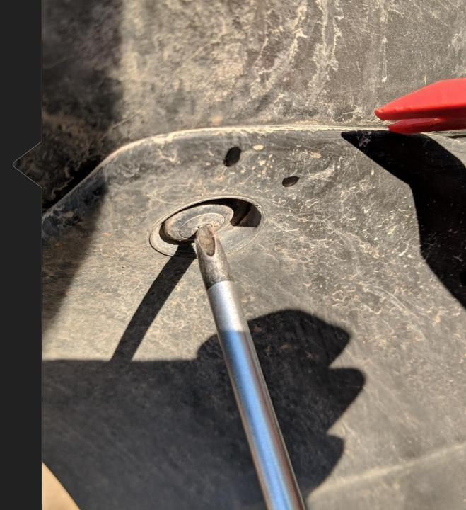
Remove the 3 plastic clips from the factory rear bumper and replace with 3 extruded nuts.
