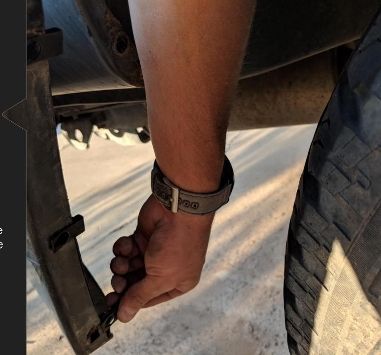
Remove the 2 plastic clips from the body and replace with 2 extruded nuts.
