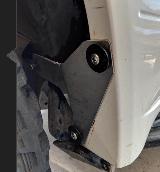
Install the 4 small allen head bolts/ lock nuts into each bracket to hold the mud flaps in place. The bolt head should be pushed snuggly against the flap then tightened into place.
