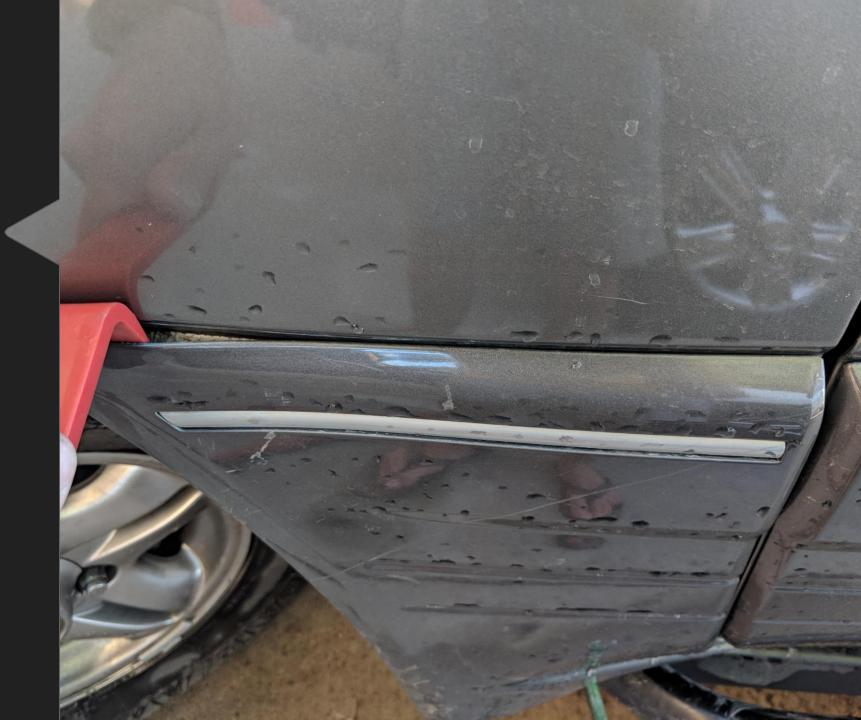
Remove only the two lower plastic clips holding the fender liner on. These often break when being removed but are not needed.
