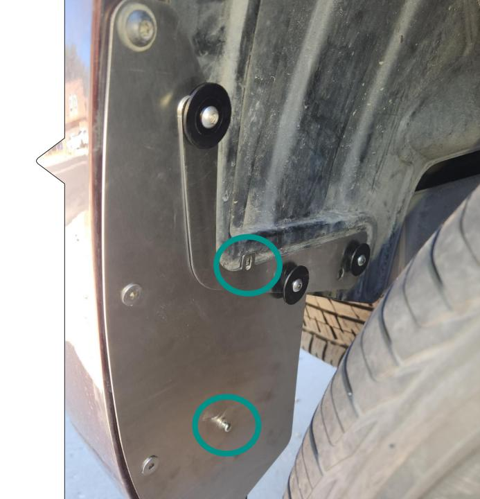
O Starting with the driver side, remove the plastic inserts in the circled holes and replace with the provided extruded nuts. These can be removed with a flathead screwdriver. The one with a finger pointing at it can be more difficult to remove. We use the flathead to break away the plastic insert while being careful not to damage the metal of the body.
