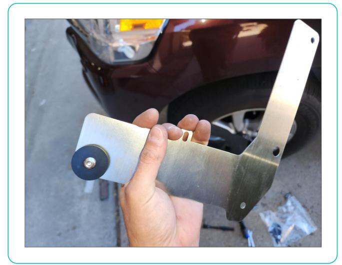
o Install each bracket using the 1" pan head bolts, washers, and spacers. In this picture, you can see we did not remove the optional plastic insert. If you did, you can install the remaining 3/4" flat head bolt at this time.
