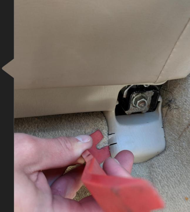
Using a 14mm socket, remove the (4) bolts holding the seat to the floor.
