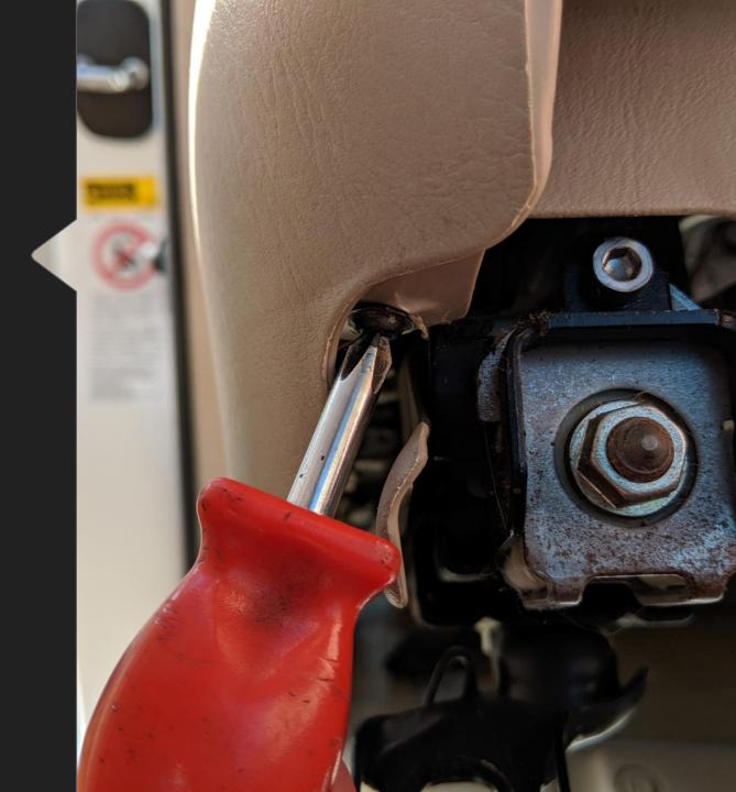
• Loosen, do not remove, the screw just below the seat adjustment controls.
