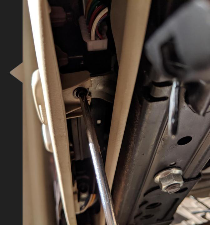
Using a stubby phillips head #2 screwdriver, gently pull back the outside trim enough to remove the screw holding the lower front trim on.
