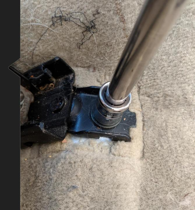
Tilt the seat backwards to make working under the front easier. You may need a counter weight or prop to keep the seat in this postiion.
