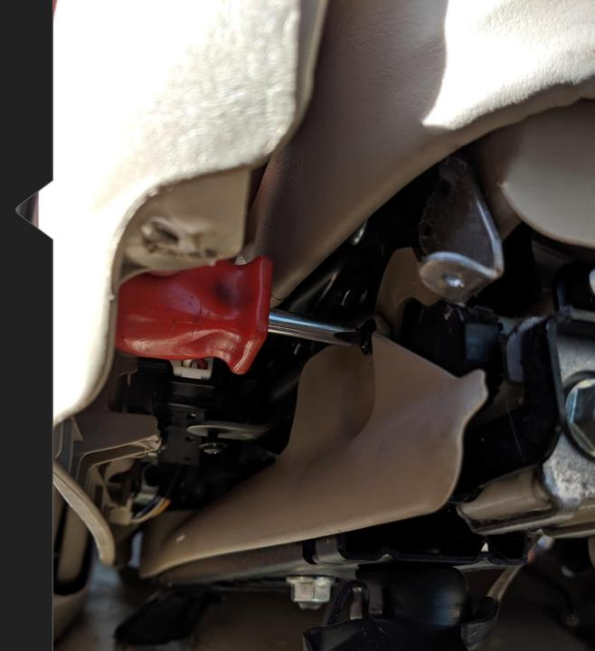
Gently pull forward the front lower trim piece. You do not have to completely remove this for installation. If you feel more comfortable removing it, repeat the previous steps for the opposite side of the seat.
