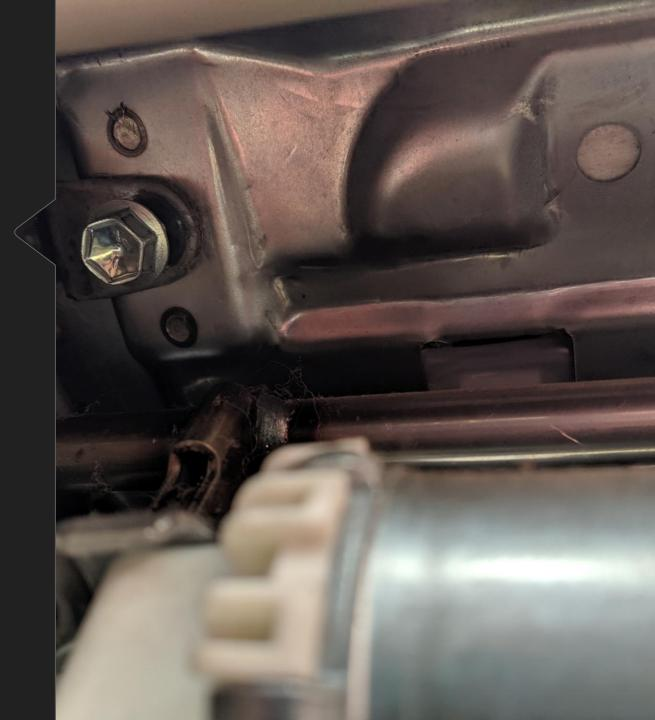
• Being very gentle of the front plastic trim, bolt your new mount using the (2) 12mm bolts removed in the last step. The bent tabs on the bracket point towards the rear of the seat.
