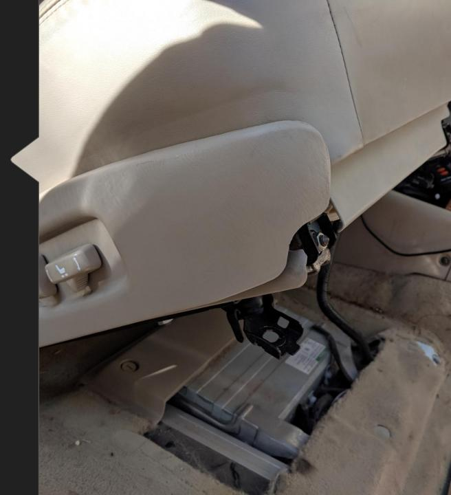
Using a #2 phillps head screwdriver to remove the plastic trim screw located at the front of the seat closest to the door.
