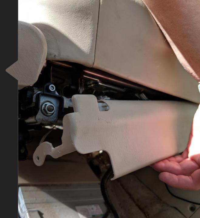
• Locate the (2) bolts located underneath the front of the edge of the seat. Using a 12mm socket with an extension, remove these bolts. Do not adjust the seat after removing these or lining the holes up will be more difficult.
