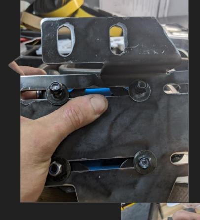
Install the bracket (with compressor for single and without for twin) using the 3 bolts provided in the kit. The larger bolts go on the top on the fender and the smaller bolt goes on the wheel well as shown.
