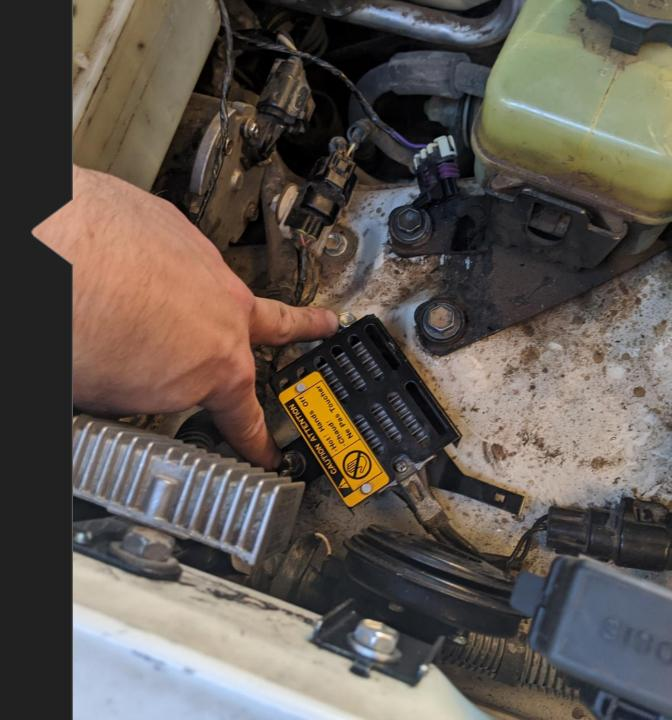
Relocate the headlight ballast to just behind where the airbox exists the fender. Use one of the bolts removed when taking it from its factory location.
