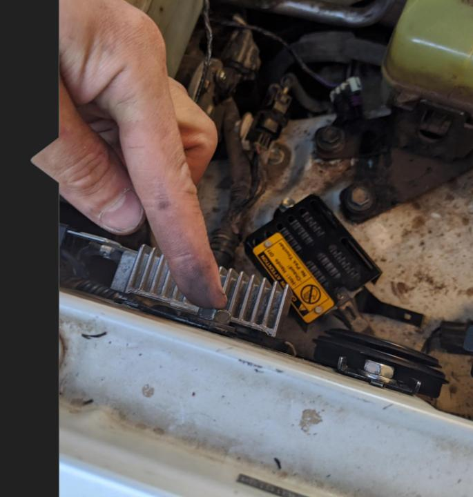
Remove the two bolts holding on the headlight ballast (if applicable)
