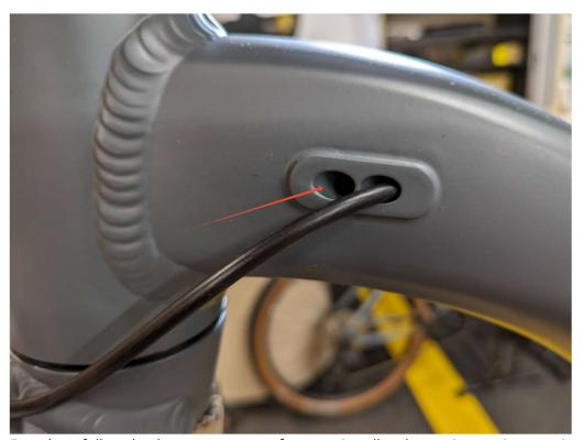
From here follow the dropper post manufacturers install and setup instructions routing the cable internally. Once the cable is routed and dropper is setup, replace the motor and bolts. Tighten to 10 - 12.5NM with a torque wrench and 6mm allen bit.
