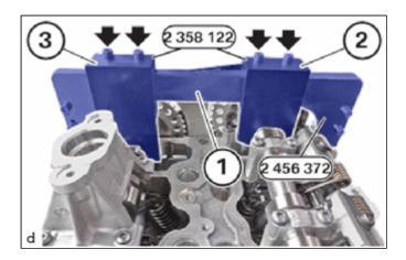
(b) Guide the test gauge (2) out of the set of special tools 2 358 122 between the intake camshaft sub-assembly and the basic carrier (1) of the set of special tools 2 456 372 and remove.
