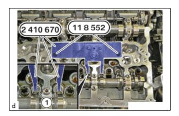
(b) Bolt in both roller cam followers (1) on the 2nd cylinder using the spindle nut of the special tool 2 410 670 up to the limit position.
