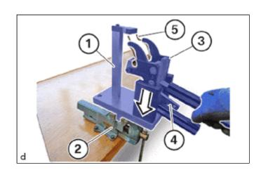
(i) Position clamping lever (3) of special tool 2 359 088 with pre-tensioned valve spring retainer (5) in direction of arrow in the mounting (1) of the special tool 2 359 088.
