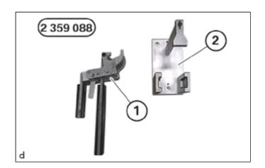
(b) Open the special tool 2 359 088 and position it at the valve spring retainer (1).
