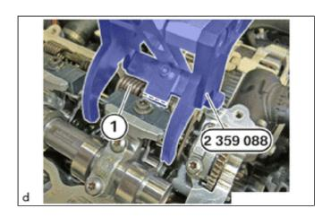
(c) Make sure that the special tool 2 359 088 lies flat against the cylinder head in area (1).
