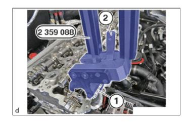
(d) Carefully close the clamping lever of the special tool 2 359 088 until the retaining hook (2) engages.
