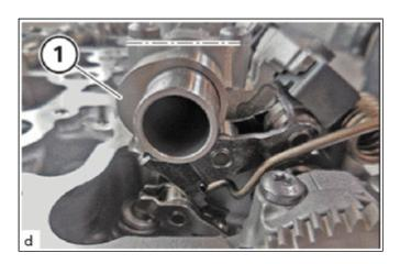
(i) Ensure that the flattened areas (1) on the intake camshaft sub-assembly and the exhaust camshaft sub-assembly point upwards.
