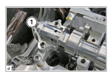
(j) Pull in all camshaft bearing caps (E1) to (E6) and the intake camshaft sub-assembly bearing cap (E) and position.
