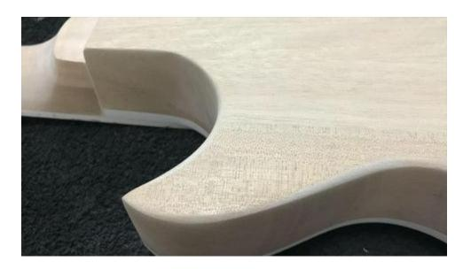
If your guitar is made from an open grain timber such as Oak or Mahogany, the open pores of the timber will prevent a flat finish unless filled. Basswood for the most part is optional. In most cases it's advisable to grain fill but if painting a solid color you can get by using a primer which will level and seal the surface.
