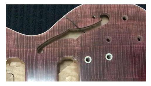
There should be a loose black ground wire in your packaging. Look for a small hole on the side of the bridge post hole nearest to the control cavity. There should be a small hole just large enough to thread the ground wire through to the electronics cavity.
