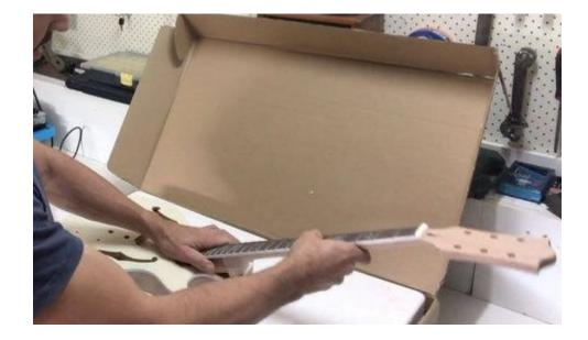
First push the heel gently into the back of the neck pocket, then push the neck down flat.
