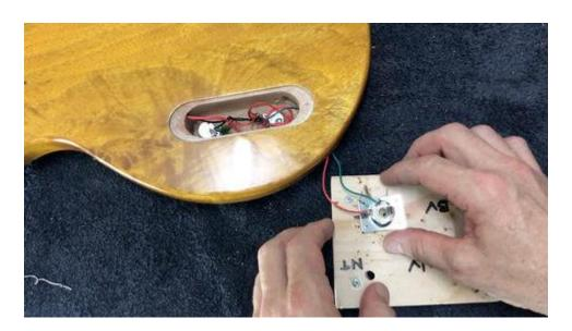
We'll need to connect the hot wire and ground wire to their respective lugs on the input jack to complete the wiring.
