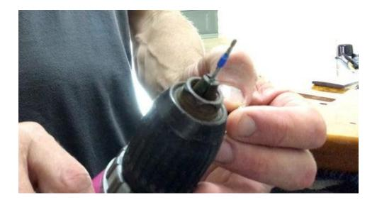
Drill pilot holes for all screws used on the body and neck of the guitar.
