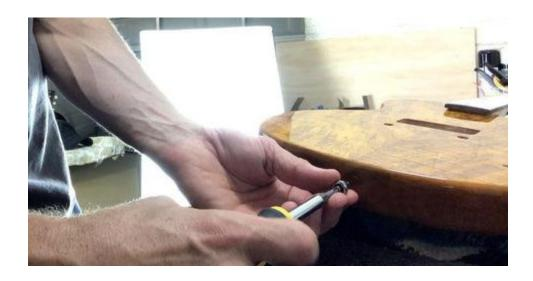
Strap buttons not only support your guitar when playing standing up, the placement of the strap buttons also affects the balance of the guitar. On an LPJ guitar, the rear strap button is located in the center of the lower bout.
