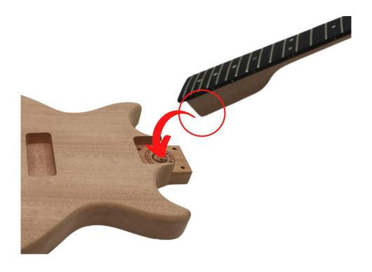
First push the heel gently into the back of the neck pocket, then push the neck down flat. This reduces the risk of chipping the thin edges of the neck pocket before the neck has been installed.
