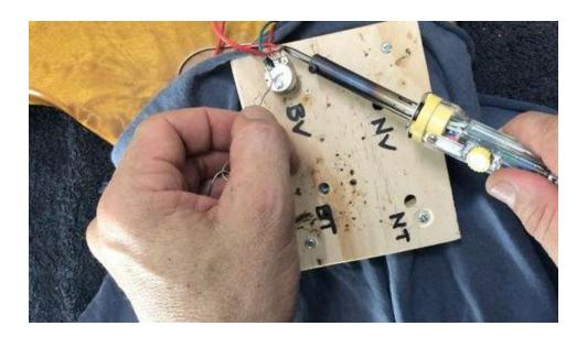
Next, take the shielded wire and connect this to the eyelet on the right side of the pot if facing away from you. Thread the wire through the eyelet and then solder in place.
