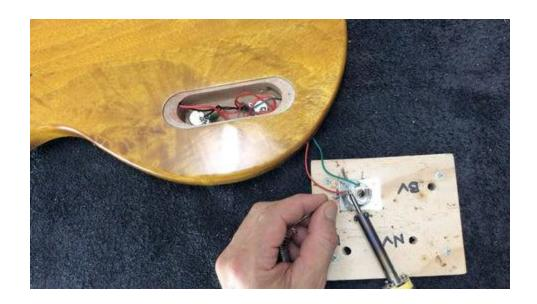
Take the ground wire from the guitar (the green wire in the image) and thread it through the eyelet of the lug attached to the inner sleeve of the input jack (the ground lug).
