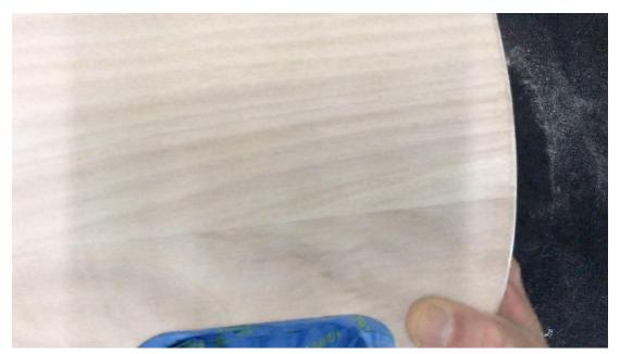
If you are staining, depending on the product you are using, you can grain fill either before or after. In most cases I've found grain filling first results in a more even application, and a better result.
