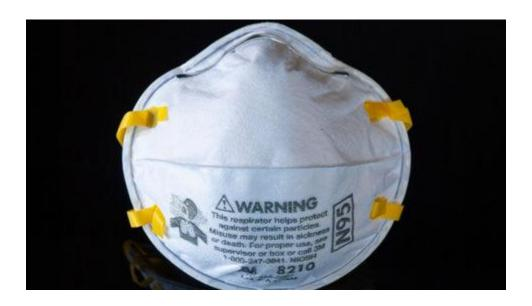
Use an N95 rated dust mask for sanding and an R95 rated particle mask for finishing. If using water based finishing products an N95 dust mask may suffice for both sanding and finishing, but be sure to check the finishing suppliers recommendations first. Paint fumes are dangerous.
