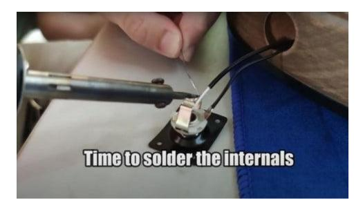
When soldering, remember to keep your soldering iron tinned, along with the components you are connecting to. Apply heat directly to the lug you are connecting the wire to until you have transferred sufficient heat to the lug, then feed some solder onto the joint.
