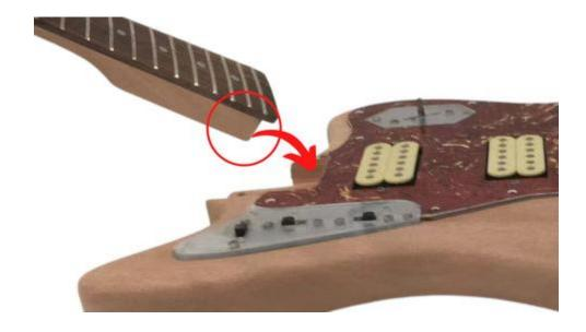
This reduces the risk of chipping the thin edges of the neck pocket before the neck has been installed.
