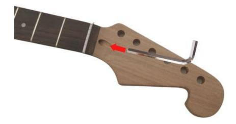
Remember to only make incremental changes of 1/4th to a 1/4 turn each time and make sure the guitar is tuned to concert pitch so the correct amount of tension from the strings is placed on the neck. Be sure to continue to check your tuning through the entire setup process.
