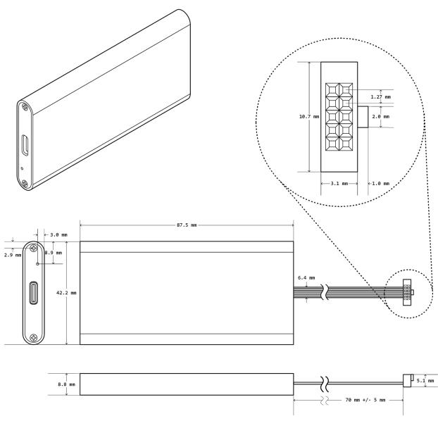
**Binho Multi-Protocol USB Host Adapter Dimensioned Drawing**
